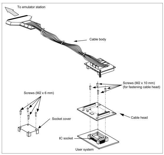
Figure 1 HS2655ECH61H User System Interface Cable
